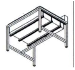
A uni-strut/all thread system works well for large sinks that will have a lot of weight in them. Please consider the application and support accordingly. Scientific Plastiscs is not responsible for damage caused by a sink not supported correctly.
