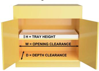
**Width-** measure side-to-side opening clearance to allow tray to slide in and out.
