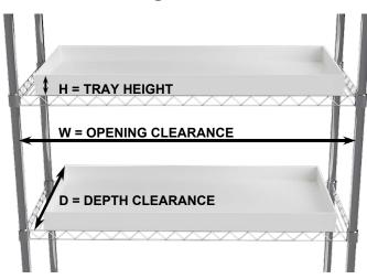
**Width-** measure side-to-side between vertical supports
