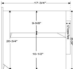
Liner designed to fit cabinets with openings 20-3/4"- 22"(H) X 47"- 43-5/8"(W).
